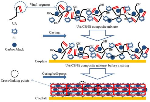
UA/CB/Si composite containing the cross-linking polymer
