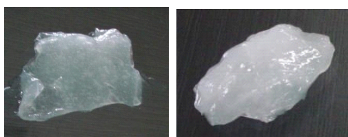
Fig. 11. Photographs of semi-transparent gel emulsion by the liquid crystal emulsification method.
