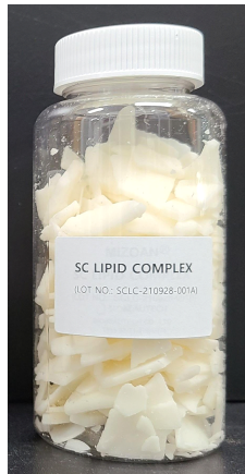
Fig. 4. Picture of surfactant of SC-Lipid Complex synthesized with hydrogenated phosphatidyl choline, hydrogenated phosphatidyl inositol, hydrogenated sucrose distearate.
