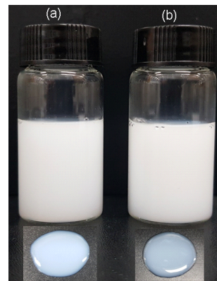
Fig. 5. Pictures of emulsifying activity using SC-Lipid Complex. a: 20 wt% caprylic/capric triglyceride, 1 wt% SC-Lipid Complex, 79 wt% water, b: 20 wt% triethylhexanoin, 1 wt% SC-Lipid Complex, 79 wt% water.
